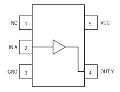
Figure 1. 5-Lead SOT-353 Pinout (Top View)
